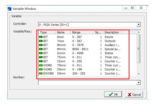
1.4.Place the corresponding variable on the HMI screen and use 485 to connect the modbus communication device, that is, you can read/write the data of the corresponding variable address, as shown in the following figure:
