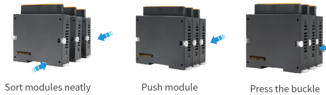
Figure 4 Snap-in buckle installation
