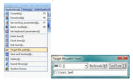
Confirm that the C drive has generated a file with the same file name and the same name as .hw6, as shown in the test program". hw6"
