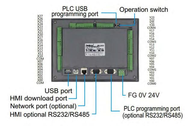
\* Dimension(mm): 226\*163\*35.6 \* Cutout size(mm): 217\*154 \* Display size(mm): 154\*87 \* Installation: Clip installation
