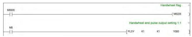
This program is 1:1 pulse output, that is, how many the hand wheel rotates, then how many pulse Y0 will output.
