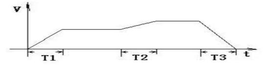
Acceleration/deceleration time T calculation= (target speed-current speed) \* acceleration/deceleration time/maximum speed.
