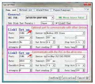
2) In Communication Parameter Settings, Open "Application --- Set Working Parameters --- Network Settings" .
