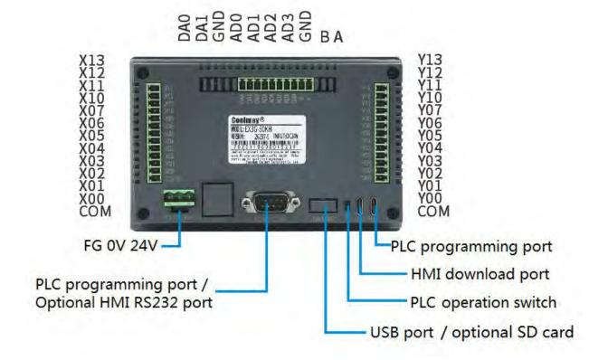
\* Dimension(mm): 151\*96\*36 \* Cutout size(mm): 143\*86 \* Display size(mm): 108\*65 \* Installation: Clip installation
