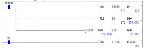
In the above figure, when M0 is closed, the value -100 is transmitted to the correction register
