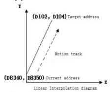
In the Center interpolation: D100 speed, D102 is the X-axis target address, D104 is the Y-axis target address, and D106 is the center X address. D108 is the center Y address. Y0 and Y1 respectively pulse the X-axis and Y-axis.
