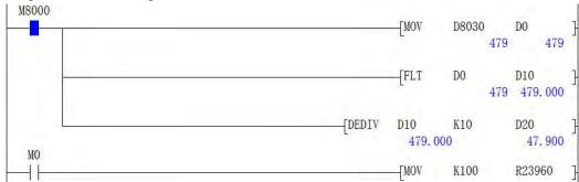
If the current temperature is  $37.9^{\circ}$ C, the actual test is  $47.9^{\circ}$ C, the error is  $10^{\circ}$ C, you need to modify the size correction register, show as below:
