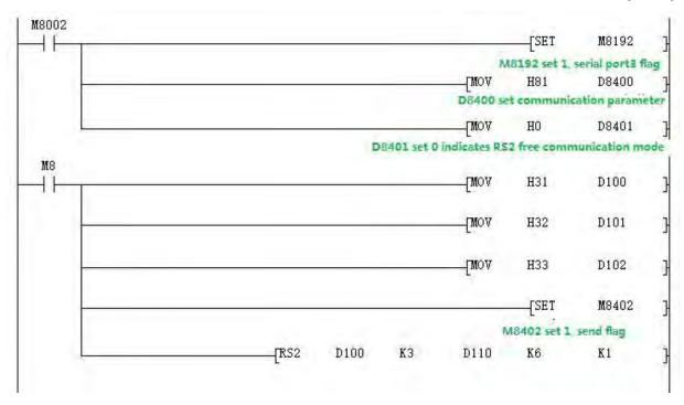
Use the serial port tool to monitor serial port 3 for data:[2017:11:01:11:49:16][receive]31 32 33 Last parameter of RS2 instruction =1: Serial port 3;
