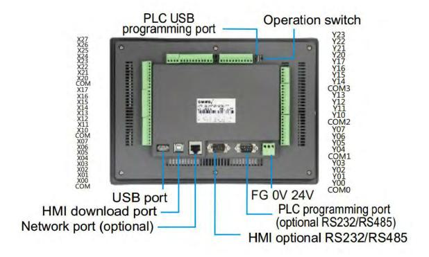
\* Dimension(mm): 275\*194\*36 \* Cutout size(mm): 262\*180 \* Display size(mm): 222\*125 \* Installation: Clip installation
