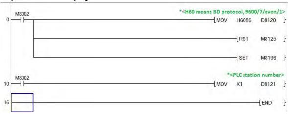
HMI can communicate with PLC by setting BD protocol master station.
