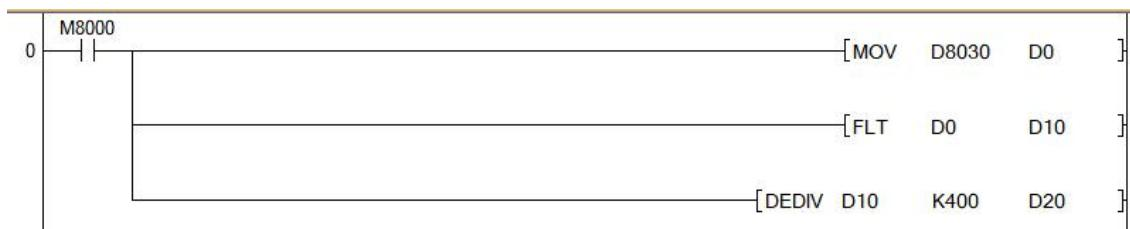
Note: When the input is 0-10V analog, the actual analog value = register reading/400;
