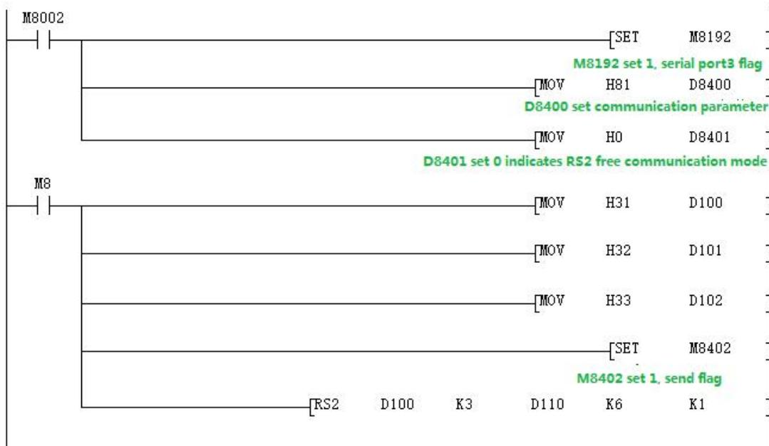
Use the serial port tool to monitor serial port 3 for data:
