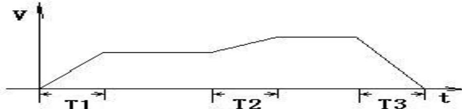
Acceleration/deceleration time T calculation = (target speed-current speed) \* acceleration/deceleration time ÷ maximum speed.
