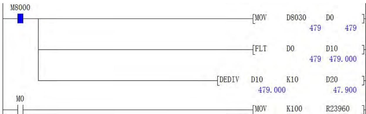
If the current temperature is 37.9°C, the actual test is 47.9 °C, the error is 10 °C, you need to modify the size correction register, show as below:
