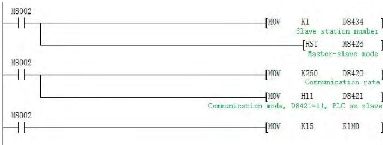
CAN port of the the PLC communicates with the CAN port of the slave PLC, and reads from the 4 bits M0~M3 of the slave PLC to the D0 of the master PLC.
