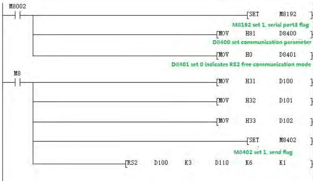
Use the serial port tool to monitor serial port 3 for data:[2017:11:01:11:49:16][receive]31 32 33
