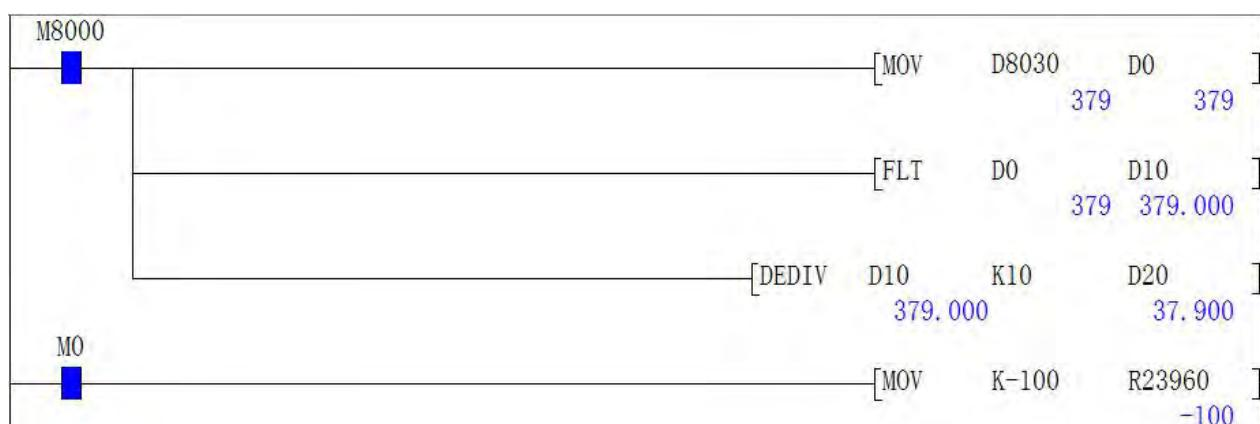
In the above figure, when M0 is closed, the value -100 is transmitted to the correction register R23960, and now you can see that the value of the actual measured temperature D20 is close to the actual temperature which is 37.9 °C.
