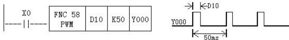
In this example, the data range of D10 is changed from 0 to 50, and the average output of Y0 is 0 to 100%. If D10 data >50, it will be wrong.
