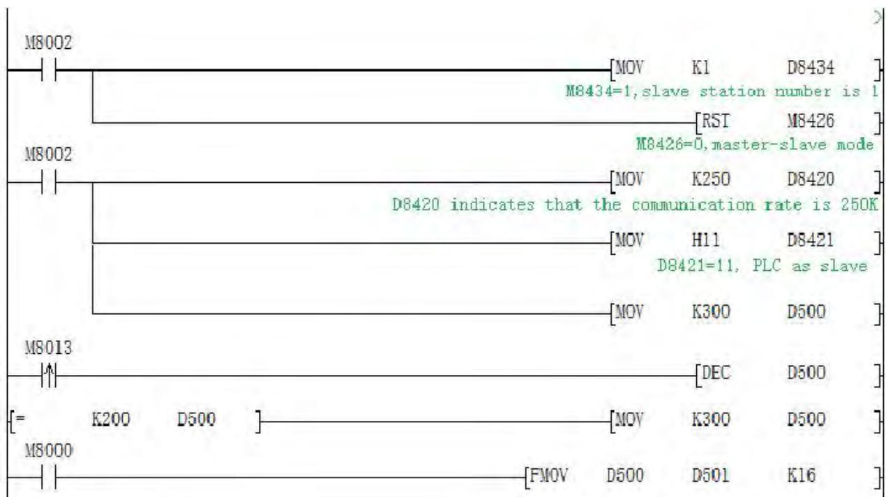
Monitoring the Master station program, the master station 16 data of D301-D316 change between 300-200 at a rate of minus 1 per second.
