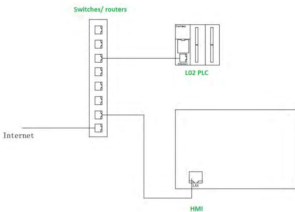
3. HMI settings (different manufacturers have different HMI settings)
