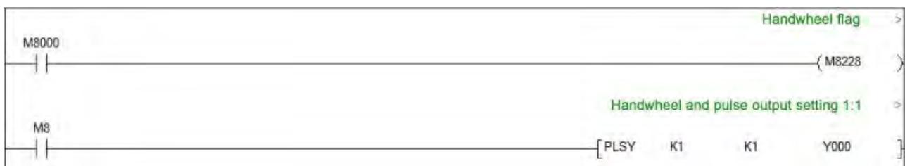
This program is 1:1 pulse output, that is, how many the hand wheel rotates, then how many pulse Y0 will output.
