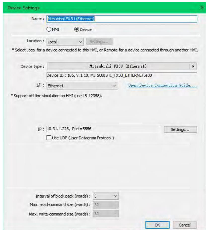
The settings in the above figure indicate that the HMI accesses the PLC whose IP is 10.31.1.223, and the port is 5556.
