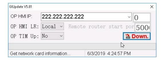
1) HMI programming software menu bar found: Tools - Network Connection Settings
